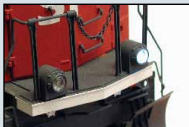
Alternating ditch lights at slow speeds
