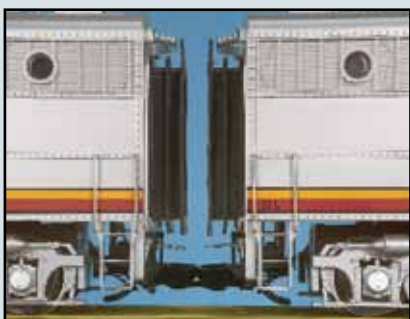
Rubber diaphragms between units
