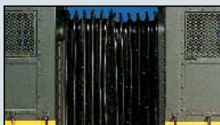
Rubber diaphragms between each unit
