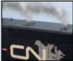
Operating fan driven smoking stacks
