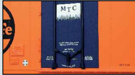
Operating plug door for prototypical opening and closing of side door
