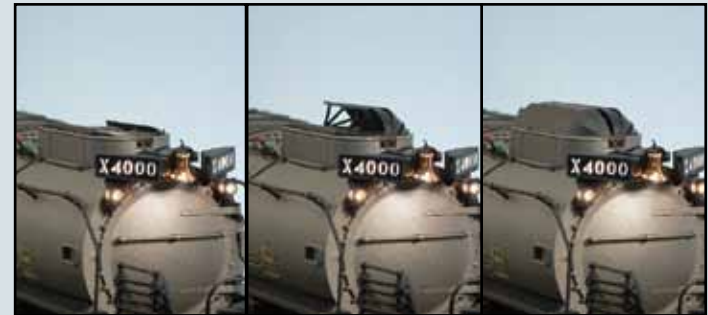
Detailed smoke deflector can be raised/lowered for prototypical operation
