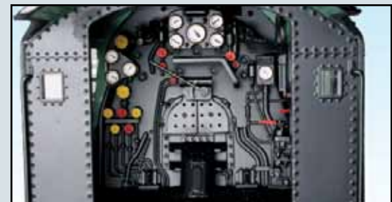
Detailed backhead including working firebox door and lighted firebox
