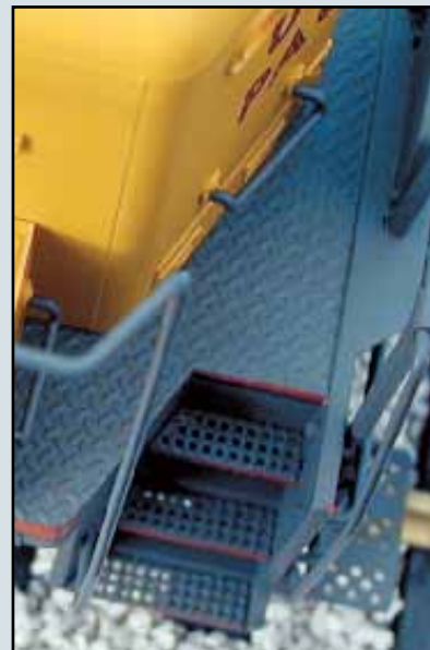
Metal Handrails and "See-thru" steps
