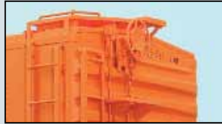
Highly detailed brake system including "real" chain
