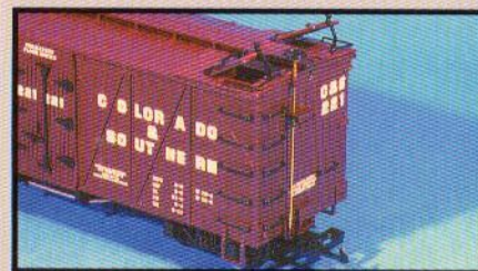
Opening ice hatches and detailed brake wheel including brake platform
