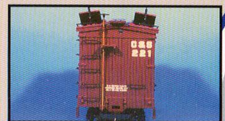
Opening ice hatches and detailed brake wheel including brake platform
